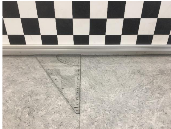
Finding a line perpendicular to the wall
